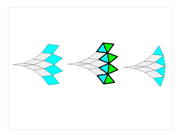
If we are constructing a rhombic fan or order m, and m is a multiple of 3, then a third of the way through the construction process we will encounter a set of rhombs with internal angles pi/3. This is a special kind of rhomb because it can be split into 2 equilateral triangles.
